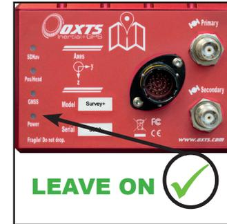
Once warmed up, system should be left on. Turning it off will require the warm up process to be repeated.
