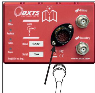
Align the Deutsch connector on user cable and socket, then twist to connect.
