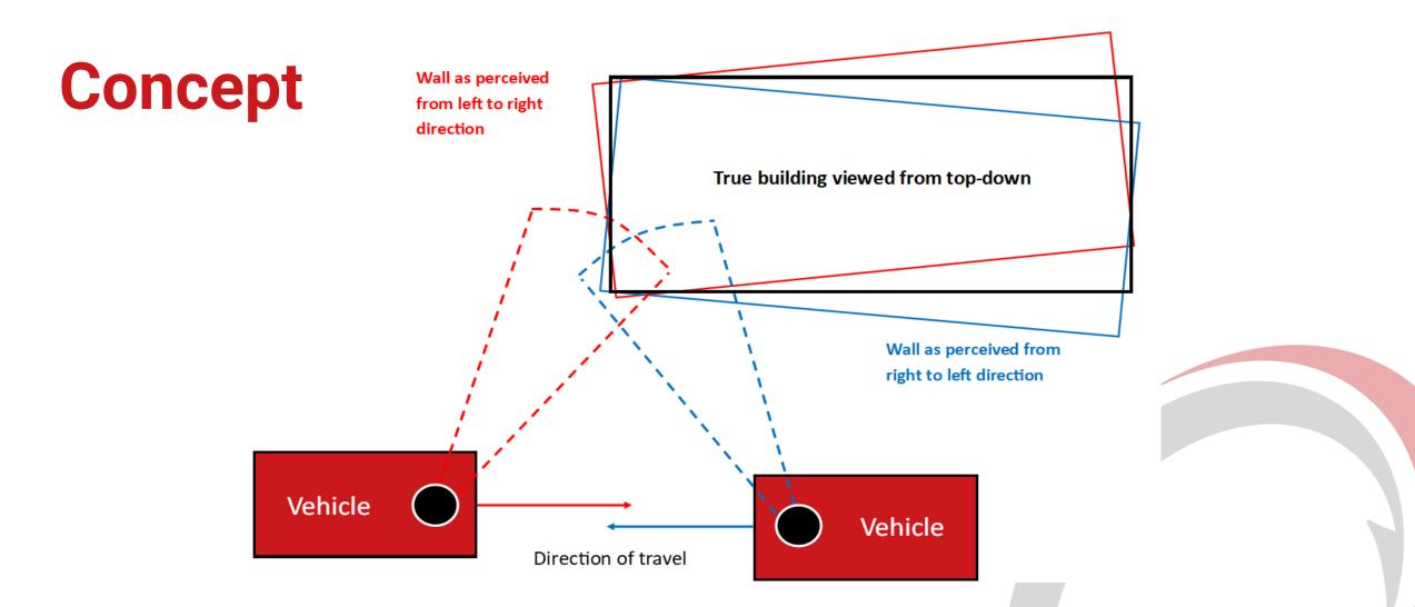
The boresight misalignment causes objects to be seen in different places when viewed from different positions and angles.
