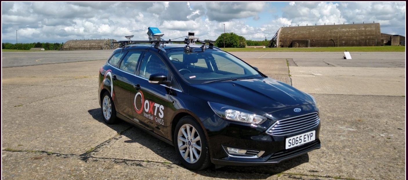
Example set-up with an INS in the boot of the car, a Hesai XT32 for LiDAR Odometry and a Z&F Profiler 9020 for mapping
